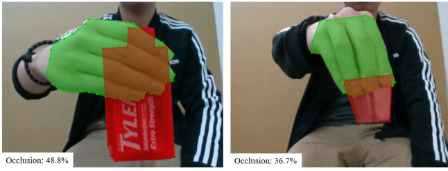
Fig. 5. Example capture of the current frame of the grasp execution for labelling hand/object segmentation and estimating the occlusion ratio.
